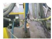
The capper requires a minimum of 80 psi to operate. Normal air pressure would usually be in the 100-120 psi range.
