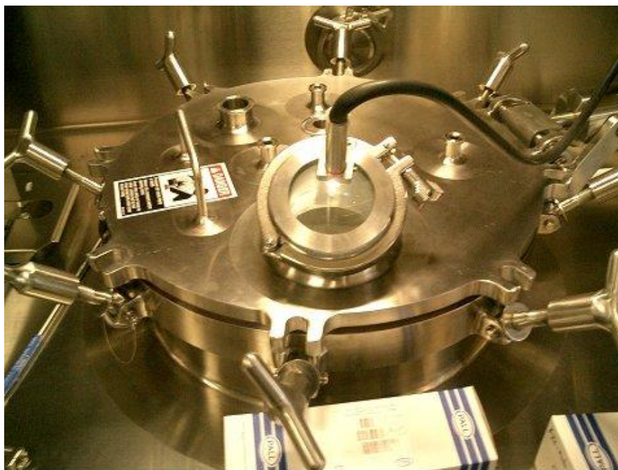
Filter with Top closed (note - not bolted shut)
