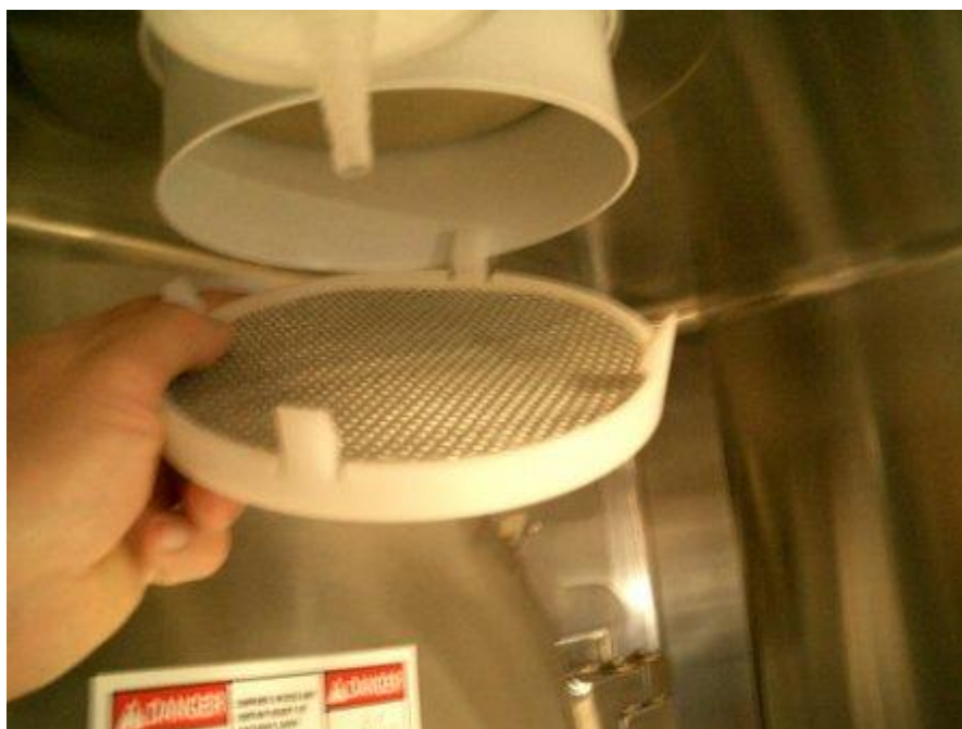
Removing prefilter from Hepa housing
